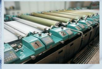
The fact is that today's rotary screen machines are highly productive, allow for the quick changeover of patterns, have few design limitations, and can be used for both continuous and discontinuous patterns. Estimates indicate that this technique controls approximately 65% of the printed fabric market worldwide.
