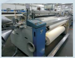
Air jet looms insert the weft yarn using air, and they enable high speed operation. The JAT 810 is the successor to the JAT710 which was the bestseller loom, and it has been comprehensively designed for greater energy savings, higher productivity and improved ease of use.
